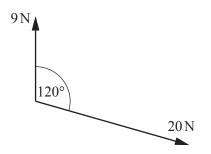
Two horizontal forces of magnitudes 9N and 20N act along bearings 000° and 120° respectively. Calculate the magnitude and the bearing of their resultant. [6]
