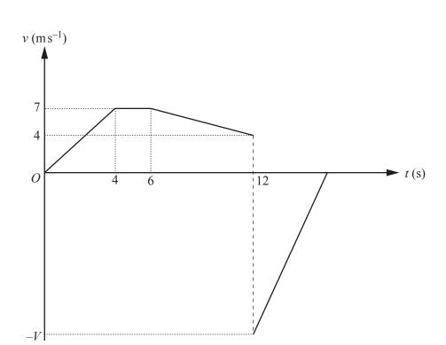
A particle *P* is released from rest at a point *A* on an inclined plane with a variable coefficient of friction. *P* descends along a line of greatest slope *ABCD*. The velocity of *P* is  $v \text{ m s}^{-1}$  at time *t* s after its release. The diagram shows the (*t*, *v*) graph for the motion of *P*. When *t* = 4, the particle passes through *B* with *v* = 7.
